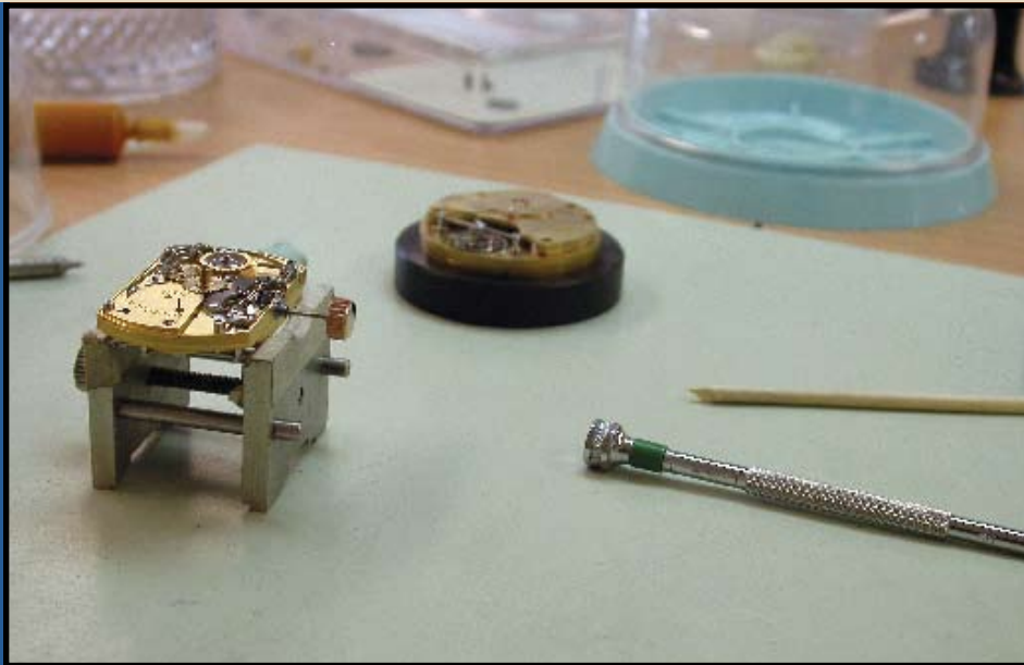
Two commissioned wristwatch tourbillons—one with calendar, one with specially calculated lunar train.
