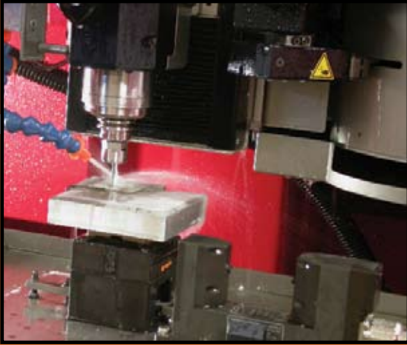
Kern milling the baseplate for the Series 2 wristwatch. Below: Francis Rossignol tweaks a commissioned wristwatch tourbillon.
