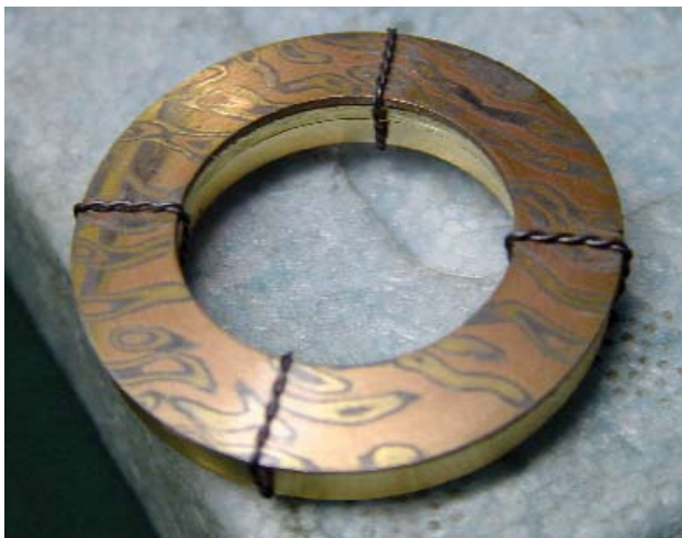
The wires on this case guarantee that the mokume gane does not move during the welding process.
