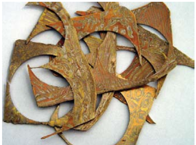
Each piece of the mokume gane made from yellow, rose and white gold is unique, making every timepiece in the series peerless.
